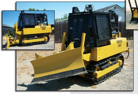
The 480 Trail Dozer is manufactured and distributed by SWECO. It is specifically designed, engineered and tested for trail-making. It is used for park and recreation maintenance; wood lots; and city, county, state and Federal maintenance work. It is also used by ranchers, contractors, military services and for fire suppression. The SWECO 480 Dozer has a 4 cylinder, 83.1 BHP @ 2500 RPM Perkins turbocharged
